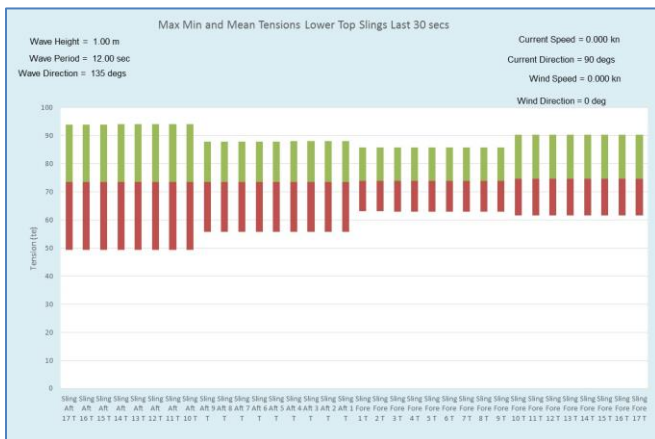
Figure 34 – Lower Steel Slings on Sewol Top Side, Sewol Depth 17m, AE=500MN, 1m Wave 135deg, T=12s
