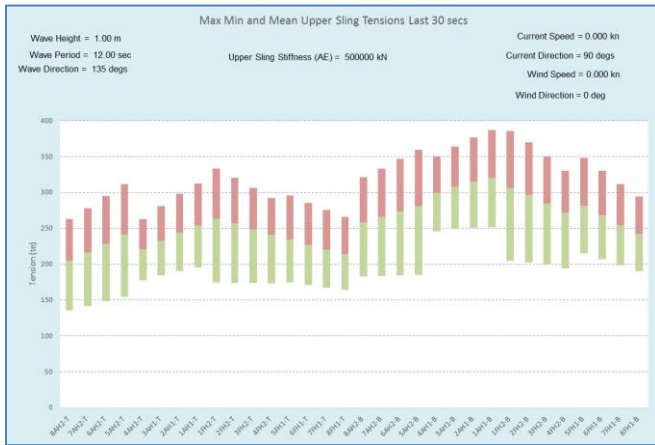
Figure 32 - Upper Sling Tensions, Sewol Depth 17m, AE=500MN, 1m Wave 135deg, T=12s
