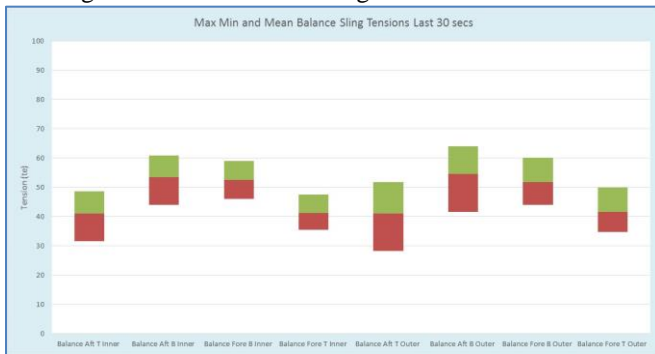
Figure 33 - Balance Sling Tensions, Sewol Depth 17m, AE=500MN, 1m Wave 135deg, T=12s
