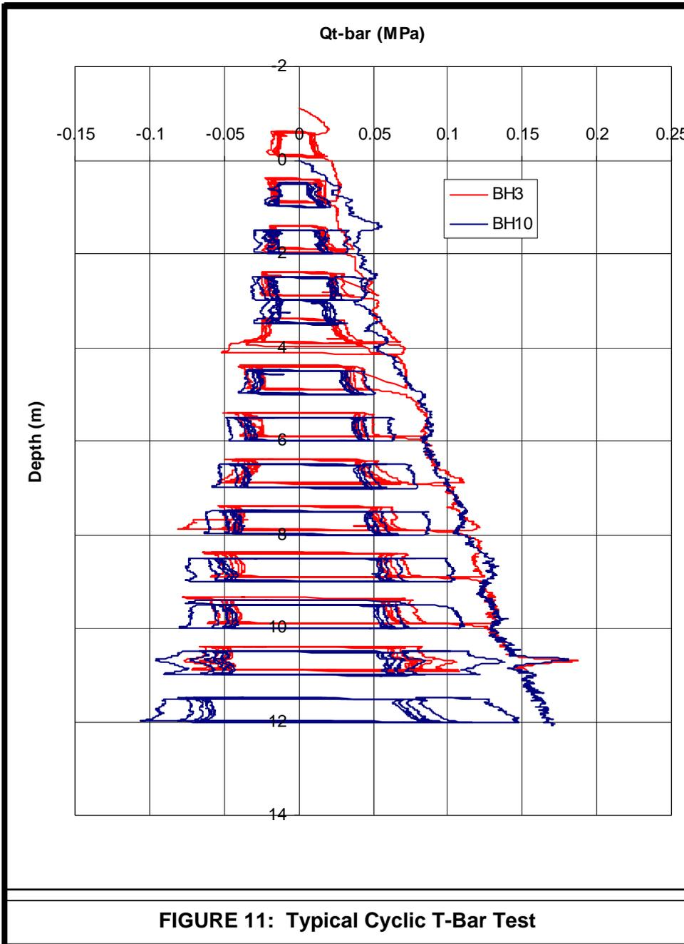
FIGURE 11: Typical Cyclic T-Bar Test
