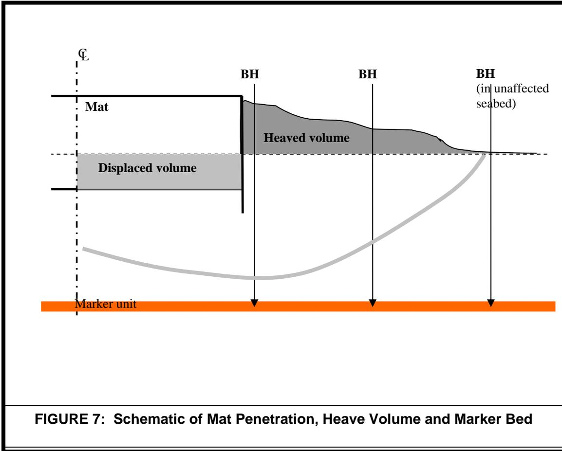
**FIGURE 7: Schematic of Mat Penetration, Heave Volume and Marker Bed**
