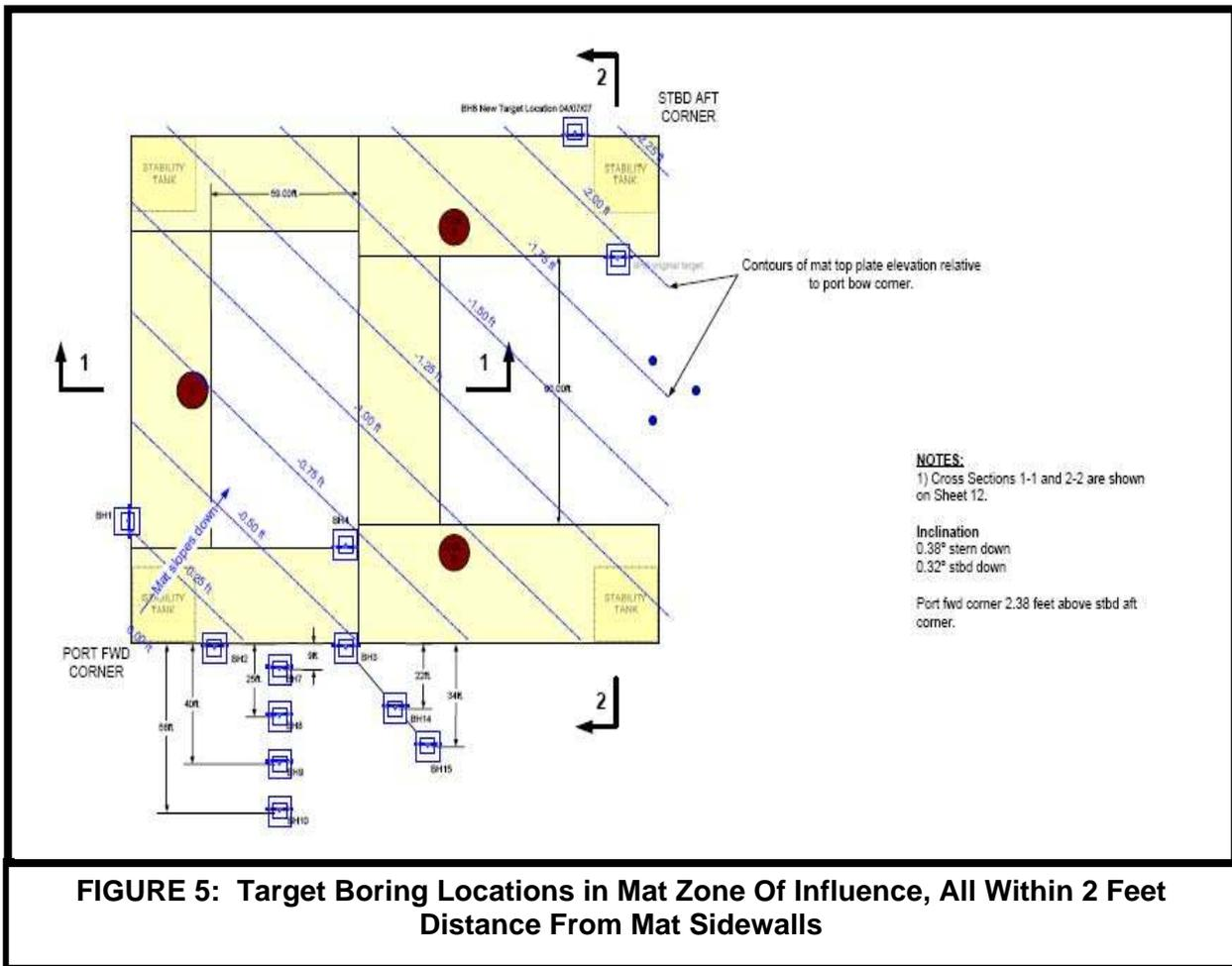
**FIGURE 5: Target Boring Locations in Mat Zone Of Influence, All Within 2 Feet Distance From Mat Sidewalls**
