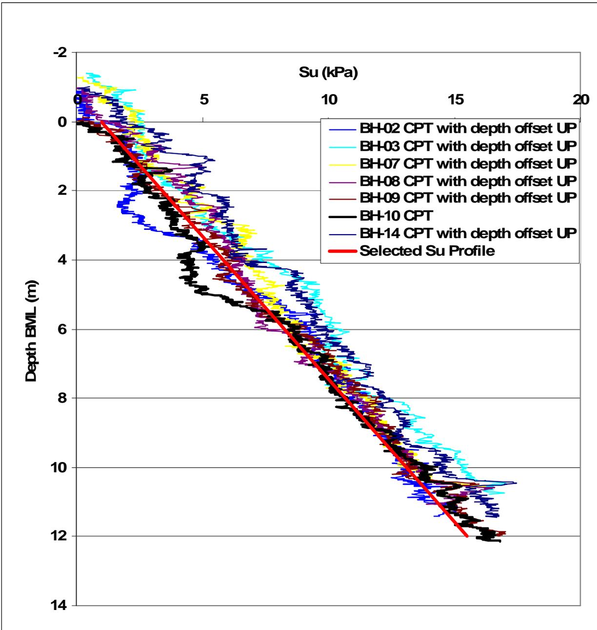
**FIGURE 9. Plot of Su Interpreted from CPT BH-02, BH-03, BH-07, BH-08, BH-09, BH-10 and BH-14 Adjusted for Common Marker Statum Depth**
