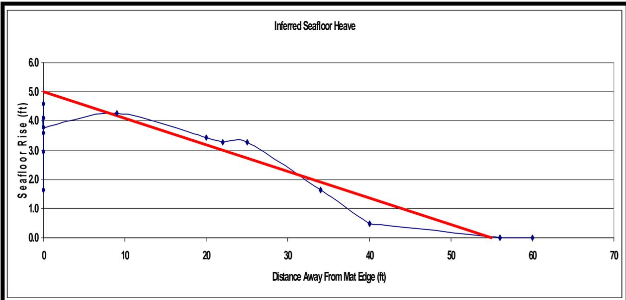
**FIGURE 8: Soil Heave Inferred from Seafloor Upward Shift Based on CPT and T-Bar Tests**
